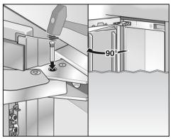
Insert the banking pin through the holes and drive in with a hammer.
